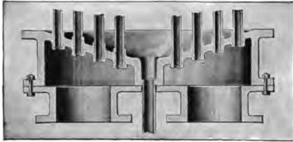
Fig. 34.—Section of Tube-plate, Bottom of Davis-Berryman Heater.
